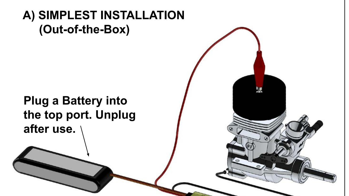
Plug the glow-plug cable into the bottom port
